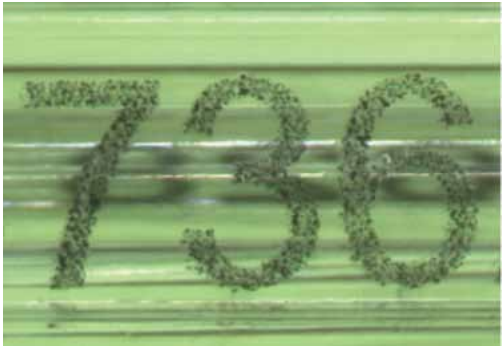
FIGURE 3. Subsurface mark in polycarbonate. Letters are 2 mm tall.
