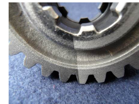
Laser Cleaning with 1 kW Pulsed Fiber Laser
