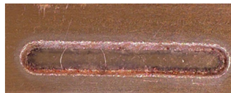
Stable and spatter-free welding of Copper contacts
