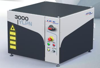
**YLPN-S Nanosecond Pulsed Fiber Lasers** offer variable pulse durations from 25 to 100 nanoseconds. The laser power can be adjusted in a wide range of pulse repetition rates independent of the pulse energy. Average output powers are up to 3 kW and pulse repetition rates vary from 2 to 300 kHz. Integrated beam switch option enables processing for multiple workstations in time or energy sharing modes.
